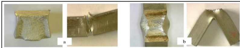
Figure 5. a. Lateral expansion of as-cast specimen in 25 °C, b. Lateral expansion of rheocasting specimen in 25 °C
