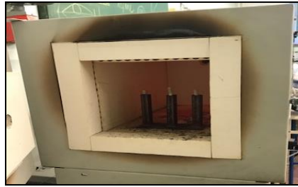
Figure 2. Melting Aluminum magnesium silicon alloys in the mold inside the furnace and The mold for the impact the samples.
