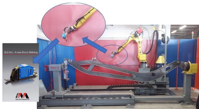
Fig. 1: Robot welding with sensor
