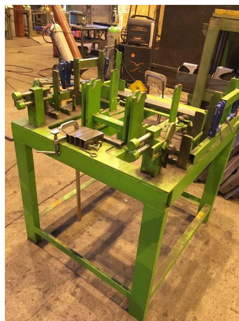
Fig. 10.: Individually designed welding jig
