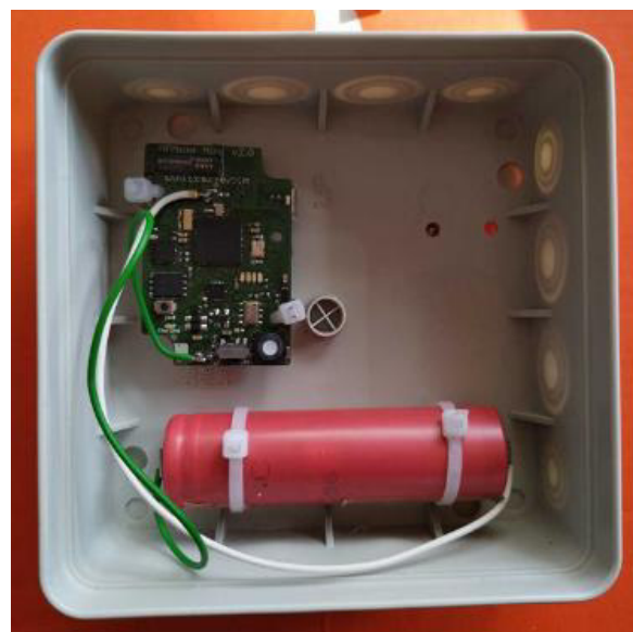
Figure 1. Sensor unit with 3 axes accelerometer
