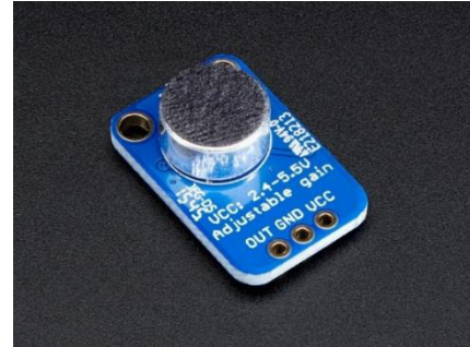
Fig. 8. MAX4466-based electret microphone with adjustable gain
