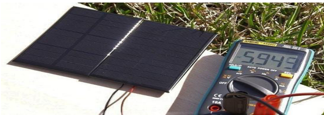
Figure-6. Measurement of solar panels with a multimeter
