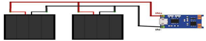
Figure-8. Connecting solar panels to the TP4056 charging module
