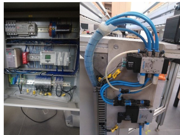
Fig. 6: Electrical cabinet of the conveyor and valve island
