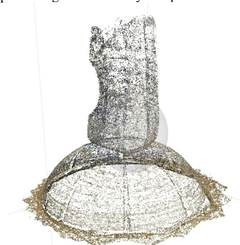
Figure 3. The point cloud model generated by automatic image matching procedure (PhotoScan)
