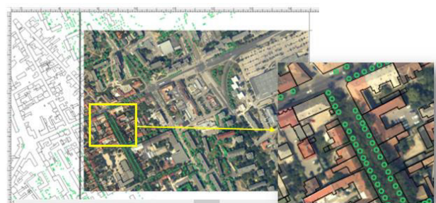
Figure 15. Cadastral map, high resolution true orthophoto and depicted individually measured trees in a common reference system
