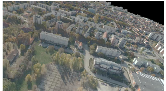
Figure 4. 3-dimensional model of Székesfehérvár by using oblique images
