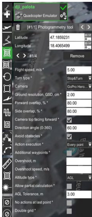
Figure 9. Setting up the photogrammetry tool parameters
