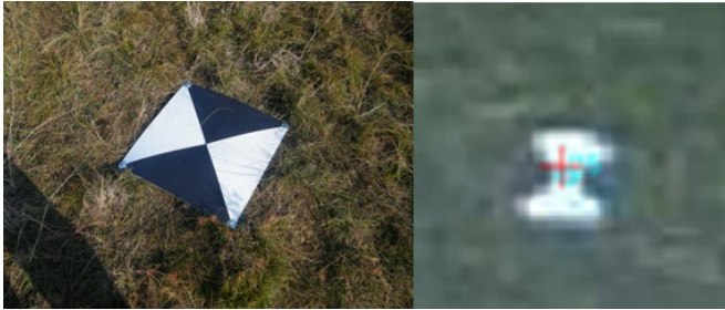
Figure 2. Ground control point sign and its image
