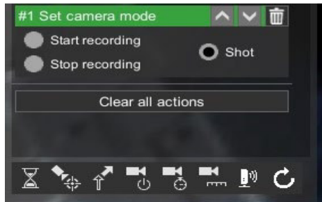
Figure 10. Setting up the camera action in each waypoint
