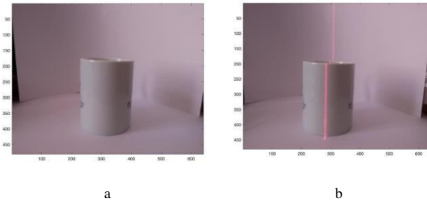
Fig. 2. Images captured using the Raspberry Pi 3 a - without Line LASER diode, b - with Line LASER diode
