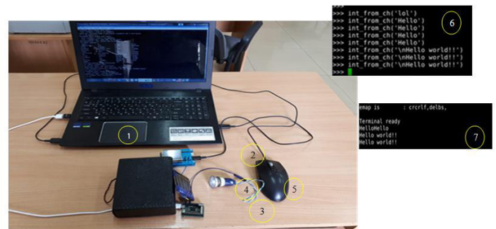
1-PC, 2,3- microcontroller STM32, 4-solar battery,5-led, 6-front panel screenshot, 7 – screenshot from the transmission panel
