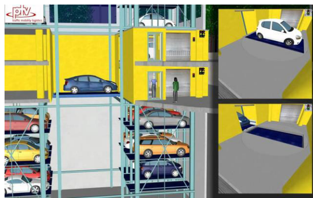
Figure 7. PTV Vissim Automated Parking Simulation [11]
