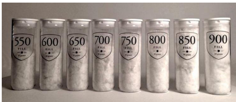
Figure 4: Fill power measuring tubes
