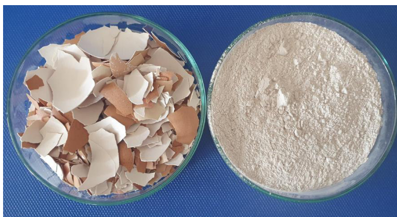
Figure 1: Eggshell waste and waste eggshell powder (ESP)
