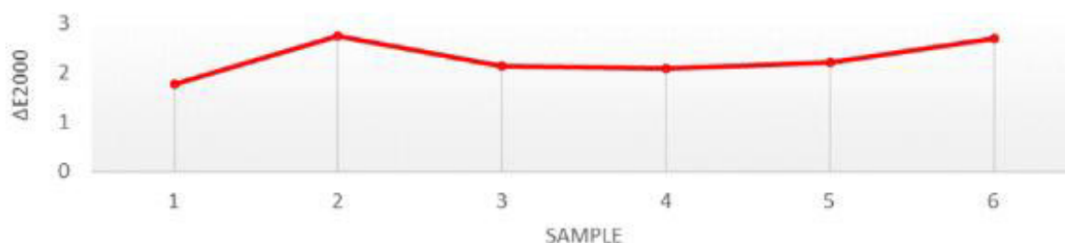
Figure 5: \Delta E_{2000} values during uncontrolled variable printing
