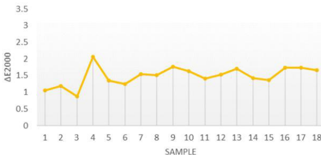
Figure 4: \Delta E_{2000} values during variable controlled printing
