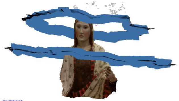
Figure 8. Madonna-head with the camera poses in two circular trajectories
