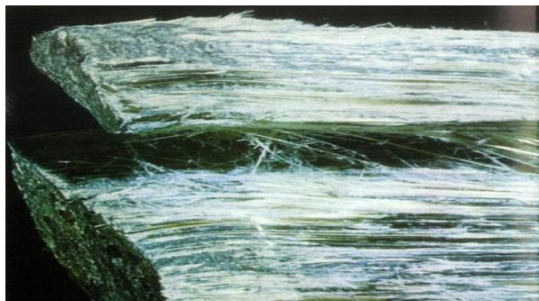
Figure 4. The electron microscope photo of amosite asbestos ( \text{Fe}^{2+}, \text{Mg})_7\text{Si}_8\text{O}_{22}(\text{OH})_2 )
