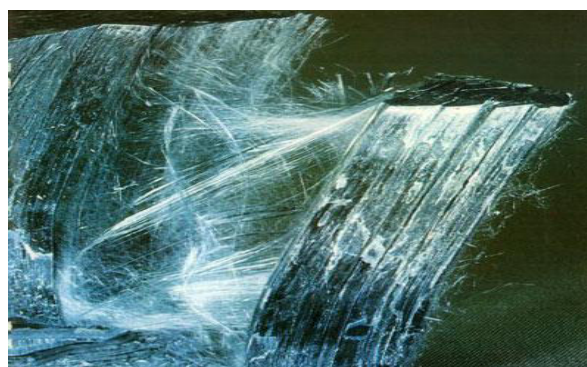
Figure 3. The electron microscope photo of crocidolite asbestos (\text{Na}_2\text{Fe}_3^{2+}\text{Fe}_2^{3+})\text{Si}_8\text{O}_{22}(\text{OH})_2
