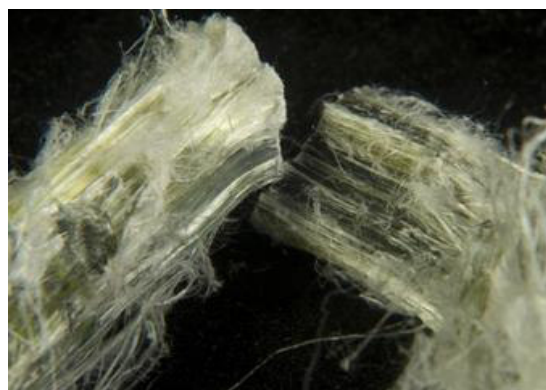
Figure 2. The electron microscope image of chrysotile asbestos 3\text{MgO} \cdot 2\text{SiO}_2 \cdot 2\text{H}_2\text{O}
