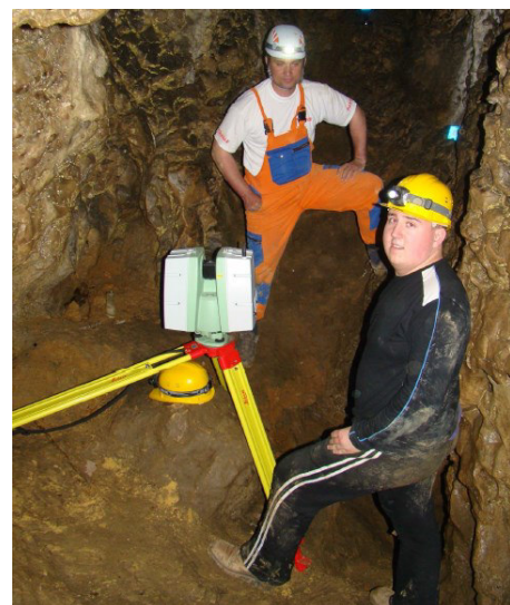
Figure 2. A laser scanner in the Cseszneki-cave
