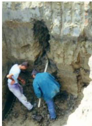
A piping's cavity level to the water side elevated. Tiszasas, no breach.
