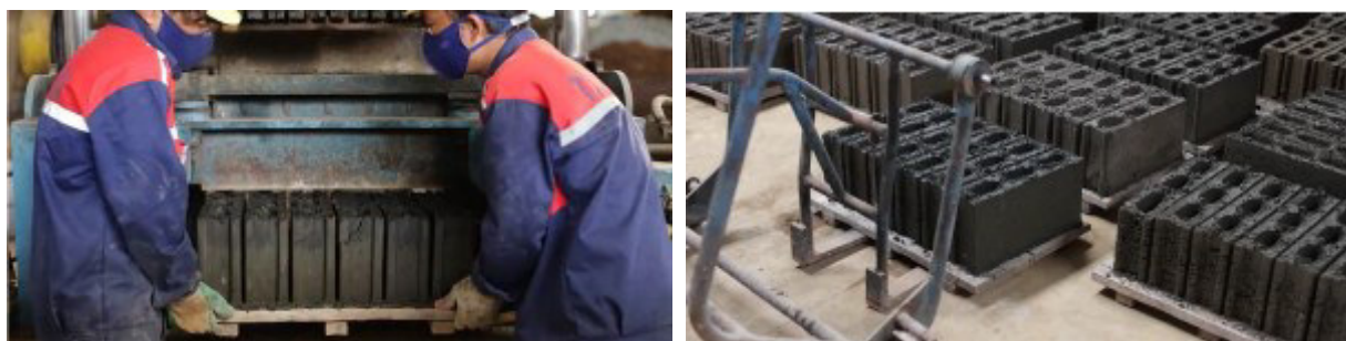
Figure 7: Bricks created by mixing the sludge, the toxic waste of the denim process
