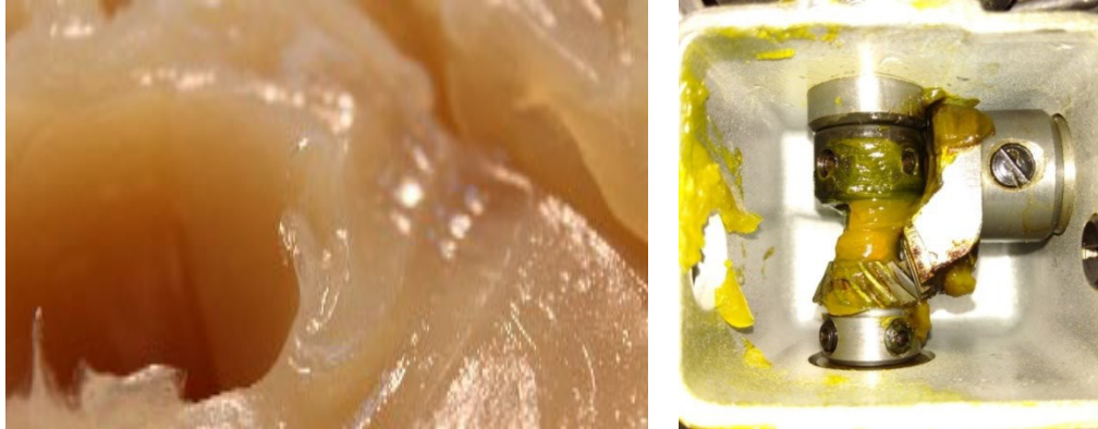
Figure 1. Grease (a) sewing machine parts lubricated with the grease (b)
