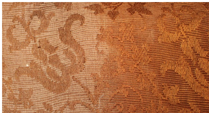
Figure 6: Discoloration of cotton fabric due to photo-oxidation
