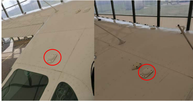
6. Figure Points of the antennas
