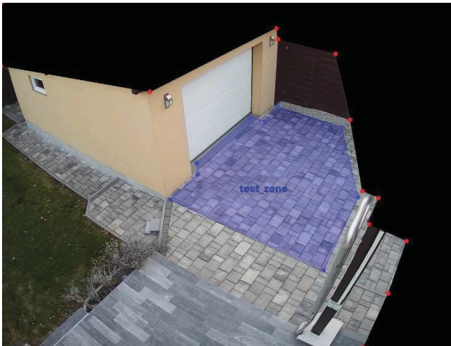
Fig. 5. Example of a motion mask and a zone named “test_zone.” Zone vertices (blue) and motion mask vertices (red) are specified by their (x, y) coordinates. The black area formed by the red vertices represents the motion mask, while the blue area formed by the blue vertices represents the zone. The image coordinate system has its origin at the top-left corner (0, 0) and extends to the bottom-right corner (2560, 1944).
