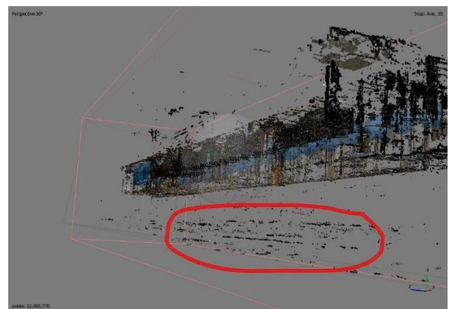
34. Figure - Noise below floor level
