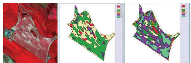
Fig. 3. Sentinel-2 image (input) and the results of two clustering procedures. The colors represent the identified clusters and do not correspond to specific thematic categories.
