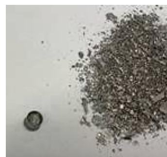
Fig. 4. Fragments of the Al–Sn alloy and pellet produced by pressing
