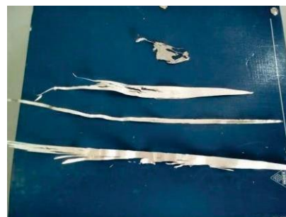
Fig. 3. Prepared metallic glass melt-spun ribbons
