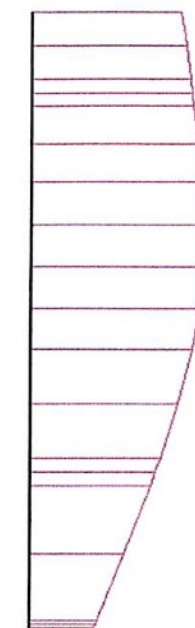
Horizontal displacements (Ux) Extreme Ux: 27,01 mm
