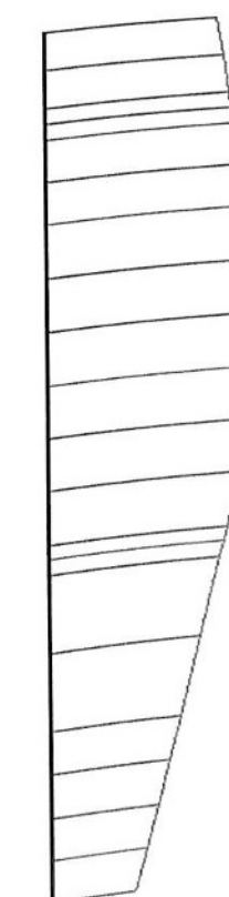
Horizontal displacements (Ux) Extreme U_x 36,38 mm
