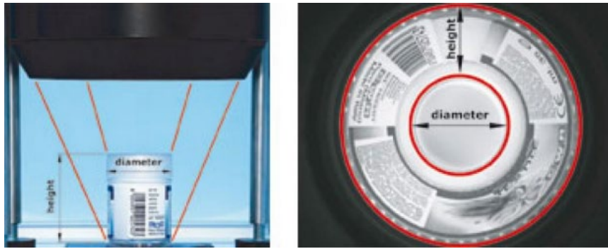
Figure 2.4: Pericentric lens' view
