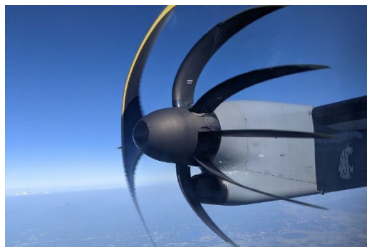
Figure 2.2: The rolling shutter effect
