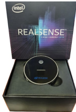
Figure 4.3: The Intel Time-of-Flight camera
