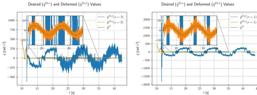
Figure 10 Deformed and desired values of the second derivative of the generalized coordinates for the multiple iterative step case (left) and the single step case (right)
