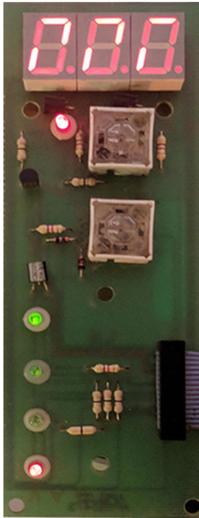
Figure 3-59: Segment Light-up test
