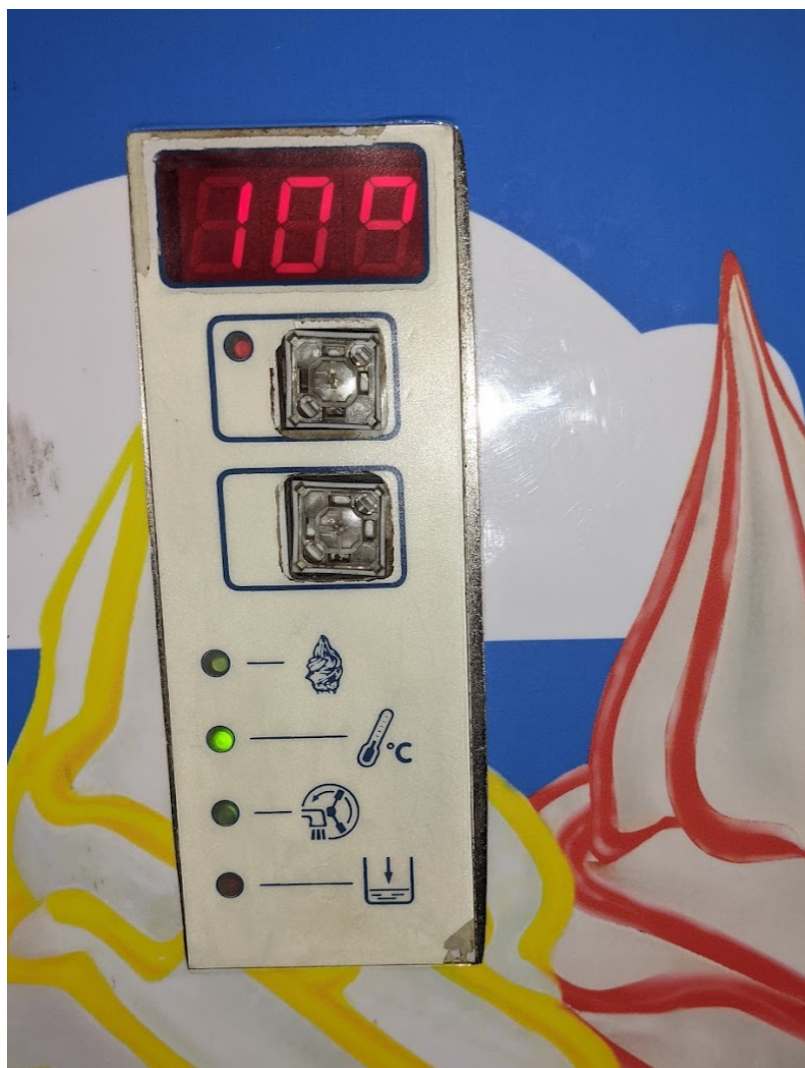
Figure 3-57: Cooling test: final temperature after settling
