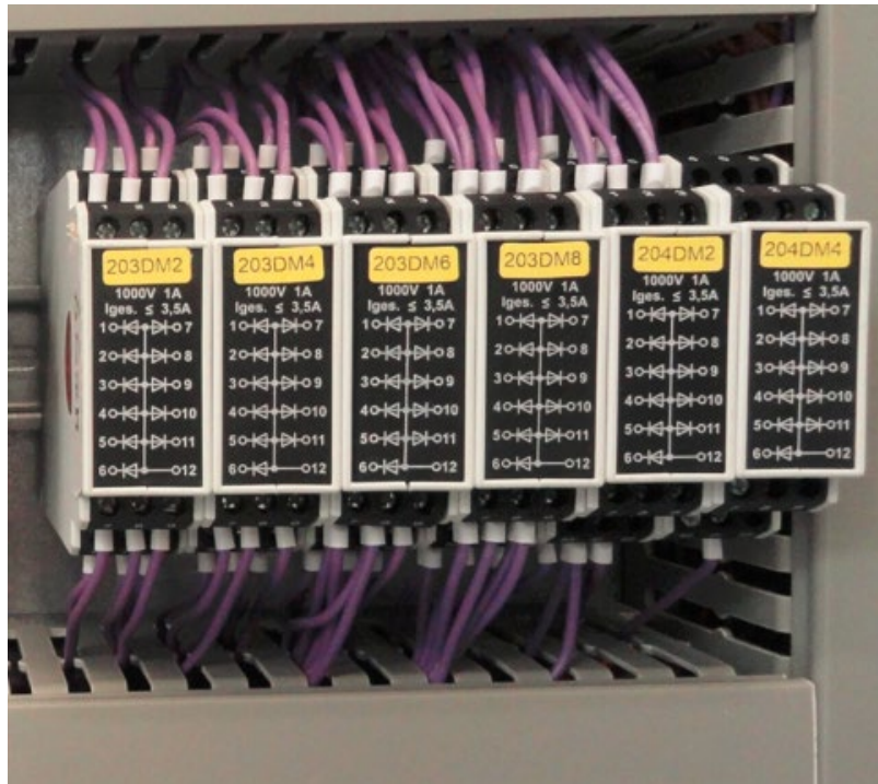
Figure 78 - Diode block responsible for LED test circuit in F2 [33]
