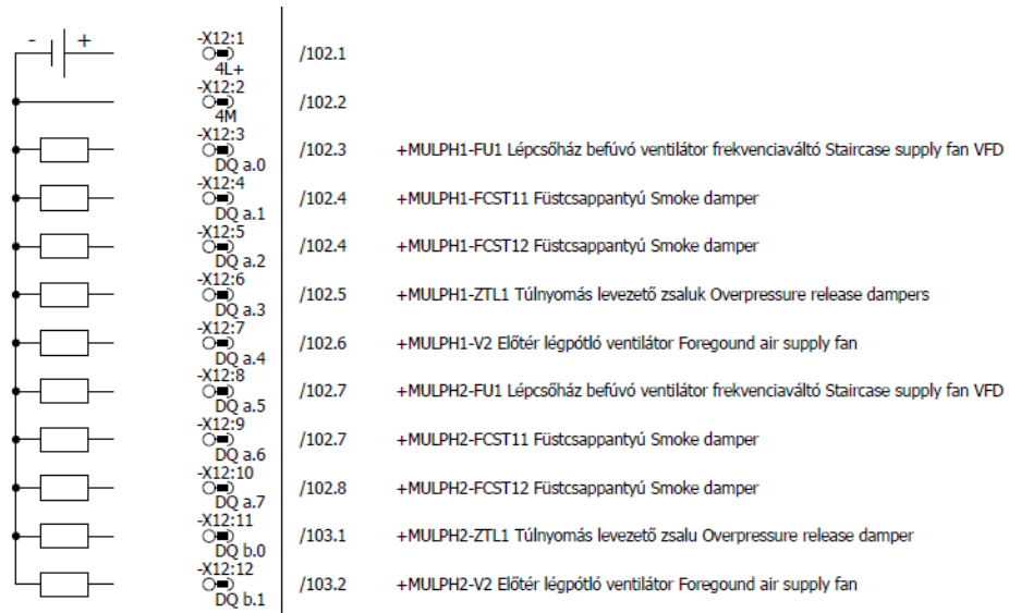
Figure 47 - Digital outputs of the PLC in F1 [18]
