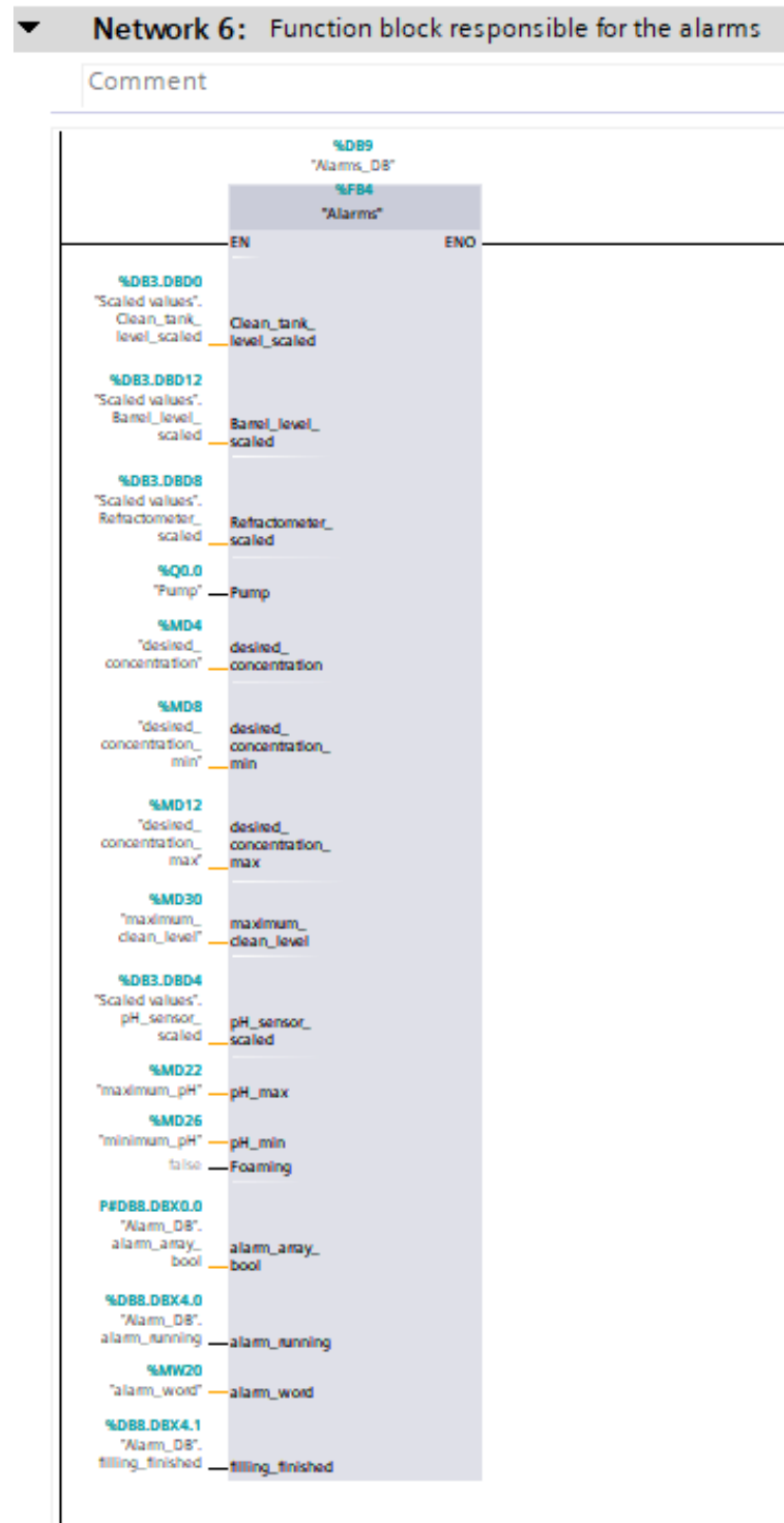
Figure 24: Alarm function block
