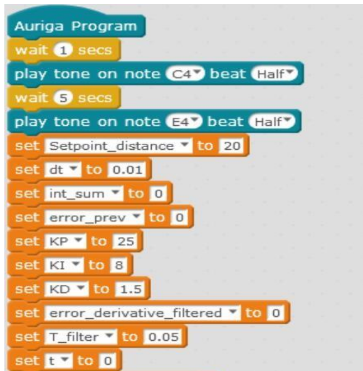
Figure 21: Graphical Programming for the PID Data Holding
