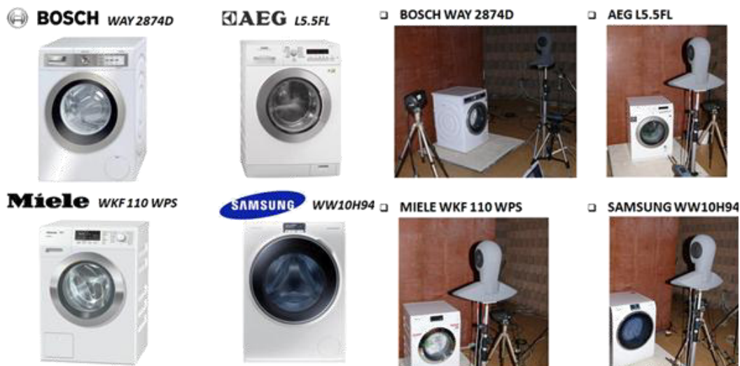
Figure 7: Measurement of psychoacoustic parameters of washing machines in a wireless chamber
