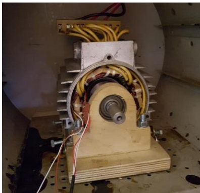
Figure 9. Experimental set with sensors inside of the furnace
