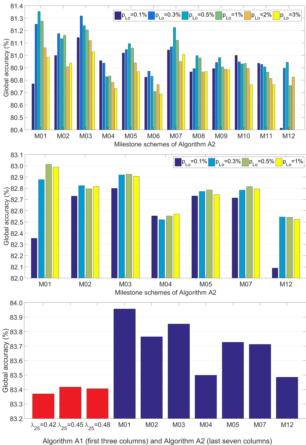
Figure 4.4: Global accuracy achieved by the random forest classifiers RF_1 (top), RF_2 (middle), and RF_3 (bottom) in the segmentation of infant brain tissues, after histogram equalization via Algorithm A2 using various milestone settings and p_{Lo} parameter values, or Algorithm A1 with various values of \lambda_{25} . RF_3 combined with Algorithm A2 used p_{Lo} = 0.5\% .
