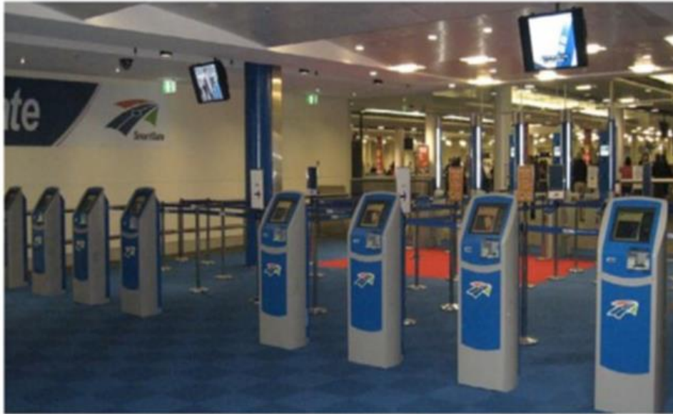
Figure 2 Photo of Smart Gates (Facial and Fingerprint) Brisbane International Airport from Frontex, 2010 [20]
