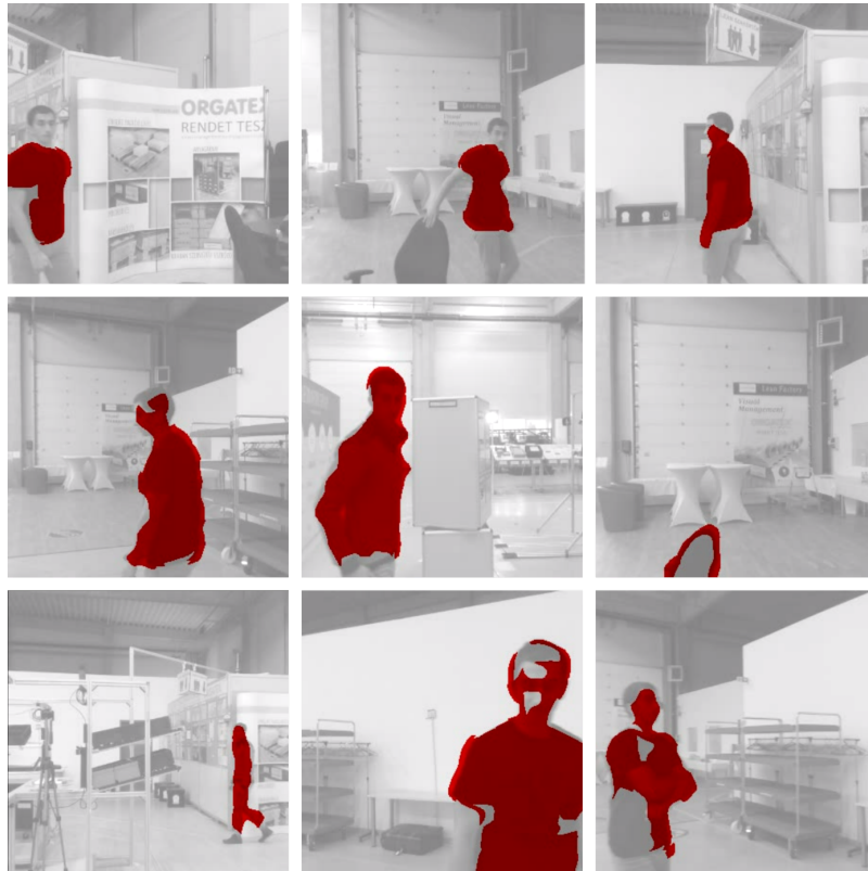
Fig. 3.5. Ground-truth segmentation masks generated by the uNLC method for the FieldData set
