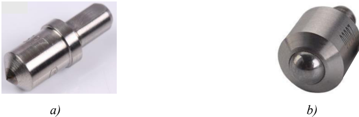
Figure 2. The standard Rockwell diamond stylus (a) and the novel steel ball stylus designed and applied in the experimental work
