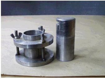
Figure 5. Reinforced crushing pot designed by Lőrincz [3]
