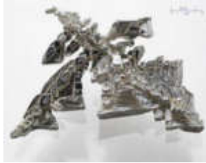
Fig. 7. Surface of bulk tin that shows typical dendritic crystallization structure obtained at a relatively low cooling rate, [9].
