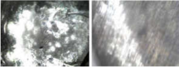
Fig. 6. For convenience and visual comparison we give two surfaces corresponding to a normal solder joint resulting from low cooling rate in open air, [op.cit].
