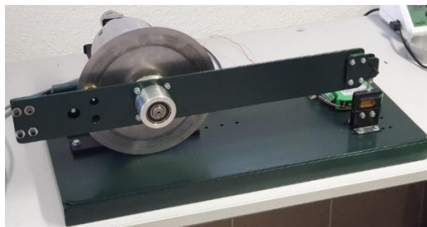
Figure 8. Test bench for the precision drive units
