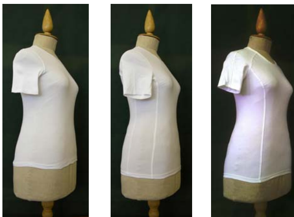
12. Figure: T-shirt with overlapping stitching and without stitching
