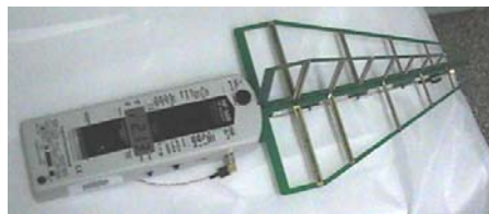
Figure 6: HF 58B Electro smog measuring set-up
