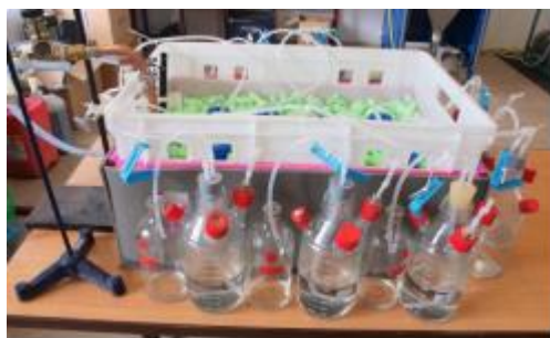
Figure 2. Insulated reactor block [5]
