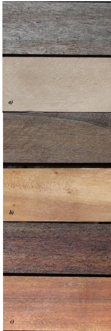
Fig. 3. The colour change of Poplar during outdoor weathering (lower: initial condition, upper: after 12 months exposure) a) Poplar control; b) Poplar 160°C/2h; c) Poplar 200°C/6h
