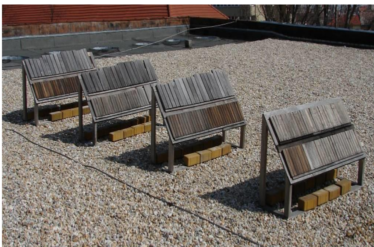
Fig. 1. The samples for outdoor exposure fixed on the stands, faced to the south, inclined by 45°
