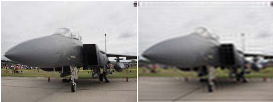
Figure 2 HOSVD-based approximation using 7500 components (left); Fourier-based approximation using 7500 components (right)
