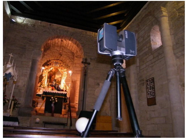
Figure 4. Surveying using a laserscanner
