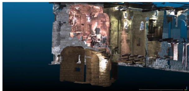
Figure 6. The upper and lower reaches of the church in a single pointcloud
