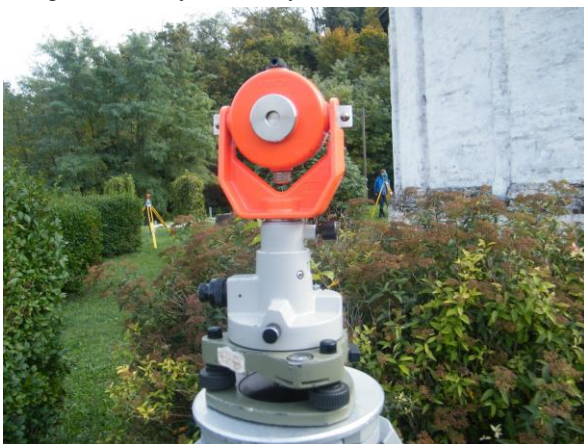
Figure 8. Measuring control point network at Kallósd church: constrain centered setting up
