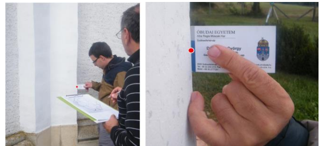
Figure 9. Measuring wall-points without prism, using card
